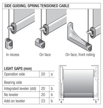
\*Size limitations and maximum load depend on operation type and are further calculated on the basis of a fabric with; weight =  $345 \text{ gr/m}^2$ , thickness = 0.44 mm. Maximum deflection of tube 31 = 3 mm, tube 37 = 4 mm, tube 50 = 5 mm.
